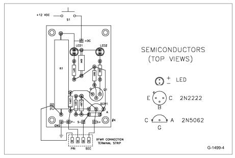
FIGURE 4: Components layout.
