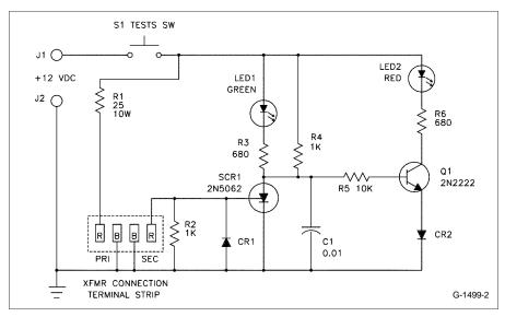
FIGURE 2: Schematic of the polarity tester.
